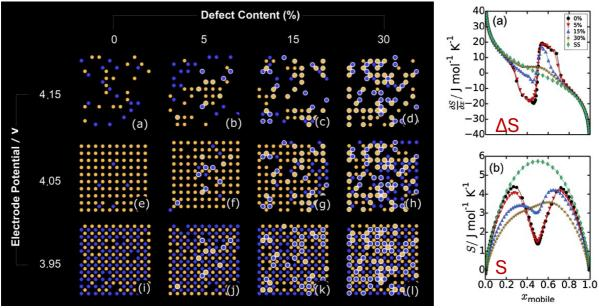
Order-disorder transitions in a spinel electrode with increasing amounts of defects: Monte-Carlo simulation of Entropy
