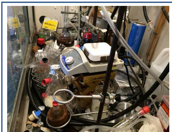
A cluttered fume hood will not have good air flow.
