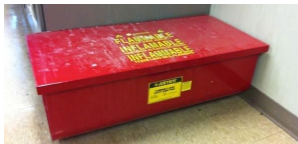
A flammables cabinet suitable for cleaning baths that contain flammable solvents.
