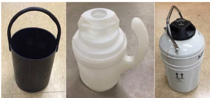
Figure 11. (left and middle) Safety carriers for transporting chemicals on campus. (At right) A portable dewar for transporting liquid nitrogen on campus.
