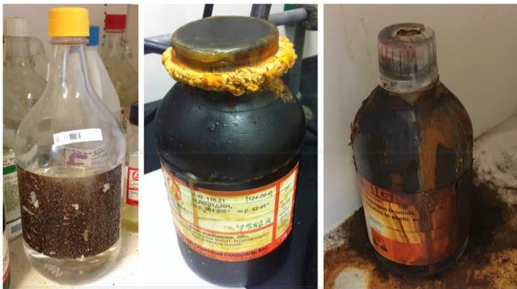
Figure 10. Problematic bottles having a damaged label or leaking caps.
