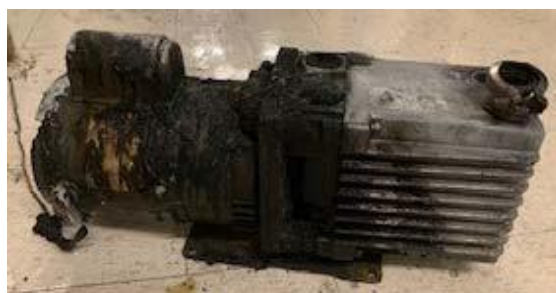
A pump that was not protected from organic vapours. https://ehrs.upenn.edu/health-safety/lab-safety/safety-alerts-and-faqs/vacuum-pump-explosion-chemistry-building
